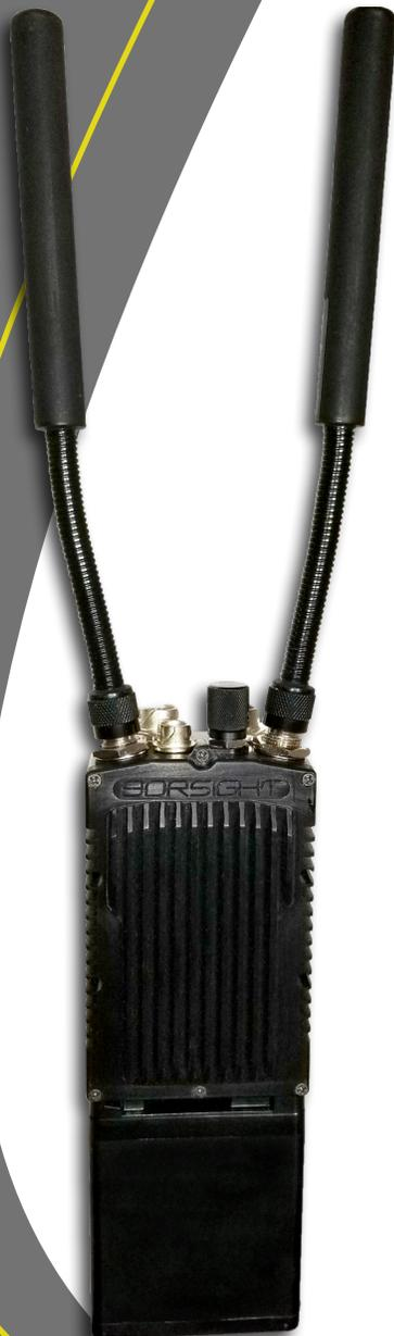
The BLOS datalink utilizes the Iridium LEO constellation allowing users to stay connected anywhere in the world with compact antennas and minimal power requirements. The LOS datalink operates in a robust ad hoc mesh network with a COFDM waveform that extends operating range and penetrates through obstacles. MIMO antennas and variable modulation modes maximize data throughput that exceeds 80 Mbps.
